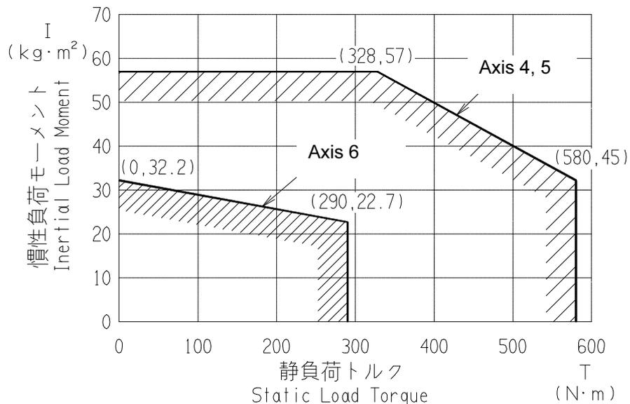
■ How to find the inertia moment of each axis
