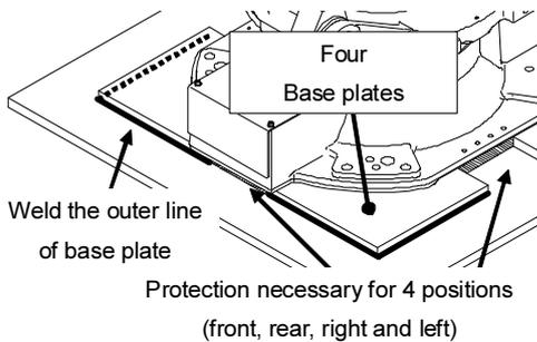
Once remove the robot and weld the inner line.
